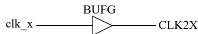
Figure 39. Spartan 3/e generation of CLK2X clock when VHDL generic clk2xen is zero
