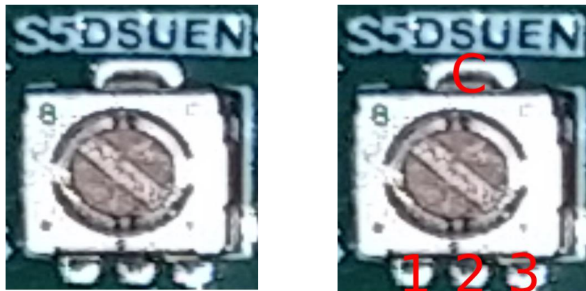
Figure 5-2: SW-SP3T mapping between schematics and a switch onboard
