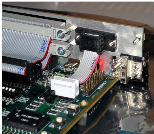
Figure 2-12: Ribbon cable connection to front Panel D-SUB connector
